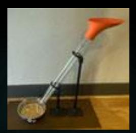
The **Dog Feeding Aid** was a 2022 student team project that allows Danny to independently feed his service dog by pouring food into a wide funnel at wheelchair height that slides down a tube into a bowl connected to the slide supported by a sturdy base.
