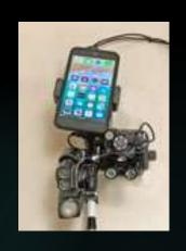
The **Smart White Cane for the Blind** is a sensor and smart vision enriched white cane for the blind and visually impaired. It incorporates a state of the art Lidar laser rangefinder, an ultrasonic sensor for object detection and avoidance, illumination for dimly lit areas, and an iPhone running Talking GPS and AIRA personal sighted assistance apps. The wheeled white cane provides contact with the surface and future guidance assistance.
